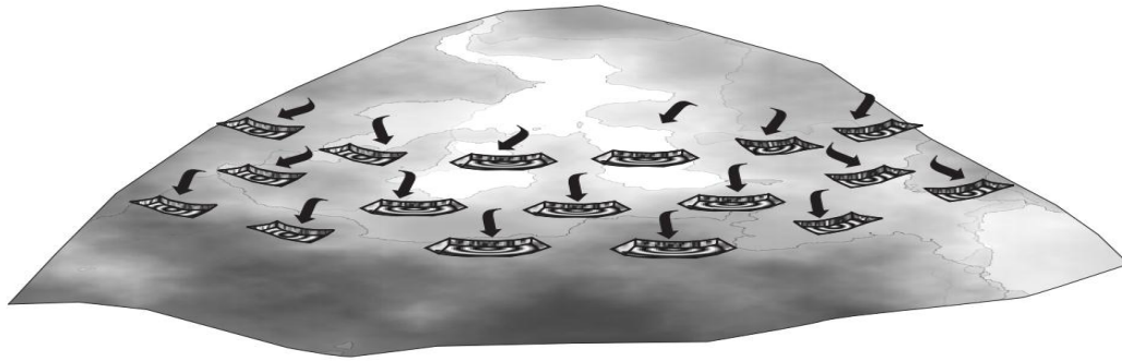
Fig.12.Staggered trenches minimise the risk of going off the contour and are therefore safer
